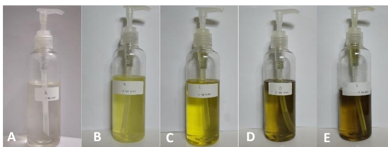
Figure 2. Liquid Shampoo Appearances (A) 720:0 (w/w) (B) 720:22.5 (w/w) (C) 720:30 (w/w) (D) 720:45 (w/w) (E) 720:90 (w/w)
