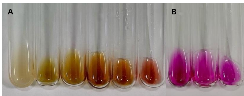
Figure 3. Biochemical test sample, (A) The test sample contains aldehydes, (B) The test sample did not contain aldehydes
