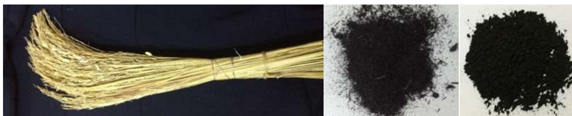
Figure 1. (a) Merang , (b) the CRS, and (c) The CRS passed through a 100 mesh screen
